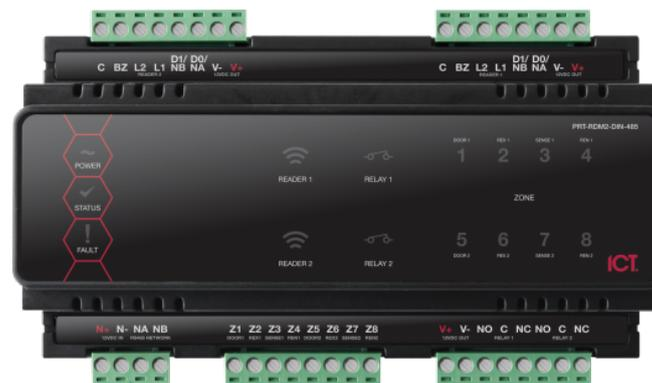
The Protege DIN Rail 2 Door Reader Expander delivers up to 4 reader inputs and 2 locking device outputs for access management in the Protege system.
